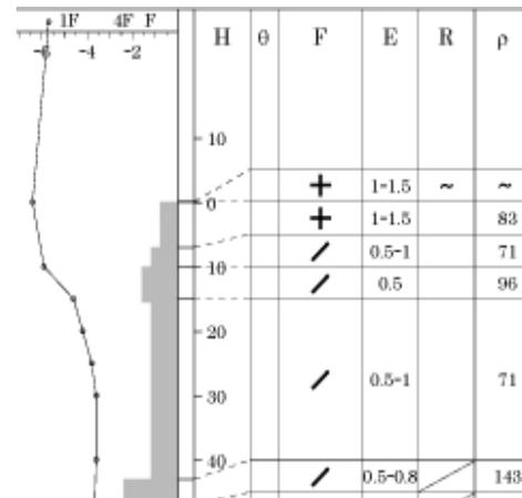
Figure 2. Temperature profile (solid line), hand hardness, snow height (H), grain type (F) and size (E), and density ( $\rho$ ) of the upper snowpack (Canadian Avalanche Association, 2007), where the toothpicks were placed.
