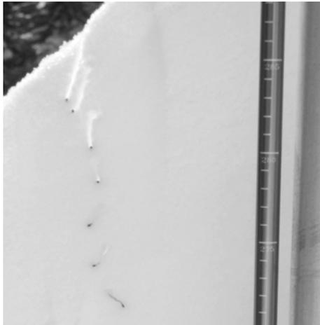
Figure 4. After 9 am the toothpicks started to melt into the snowpack in irregular patterns and were useless for creep analysis.
