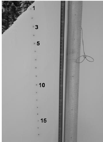
Figure 1. Toothpick profile on a slope parallel pitwall, avalanche probe as length-scale reference, and stationary aluminium post with black reference points. The profile points with numbers were selected for a more in-depth analysis.
