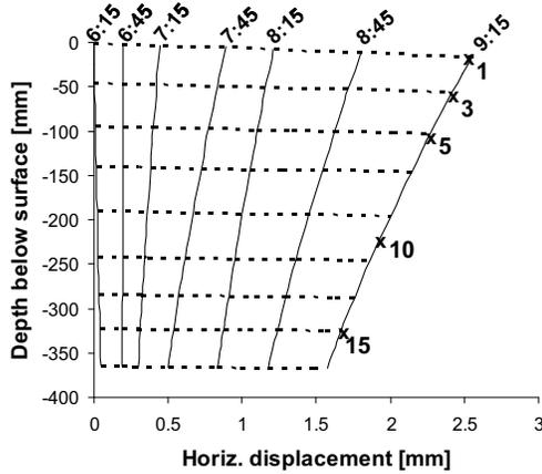
Figure 3. Half-hourly creep profiles (solid lines) and trajectories (dashed lines) of odd-numbered profile point. The numbers (1, 3, 5, 10 and 15) are selected profiles points for further analysis. Note the different scales on both axes.
